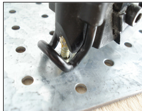
Positive nail setting. Tool fires, if nail tip lowers into the hole.
